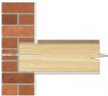
BowTie into joist end through a solid wall
