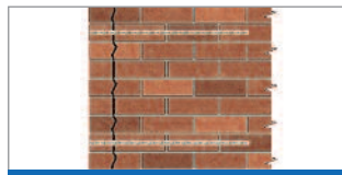
3 Repairing cracks near corners and openings
