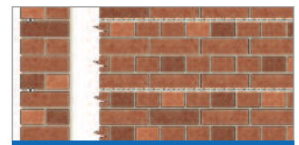
8 Creating masonry beams
